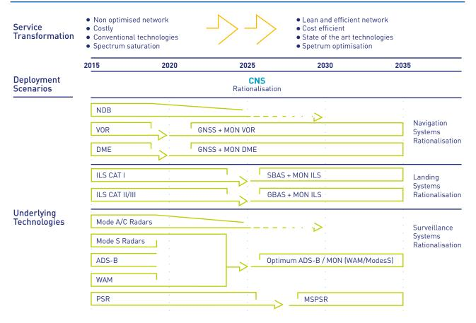
systems NDB, VOR, DME, ILS, Mode A/C/S radars, high-frequency and VHF voice, and VHF datalink mode 2 (VDL 2), by civil ANSPs, as shown in **FIGURE 13** (<sup>61</sup>).
